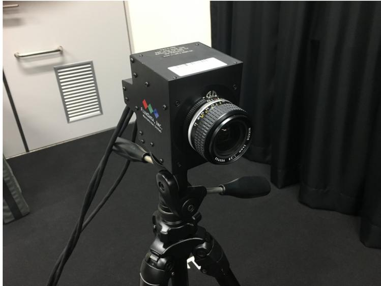
**Fig 10** Polarization camera.
