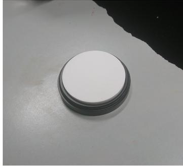
**Fig. 9** Image of the white-reflectance standard
