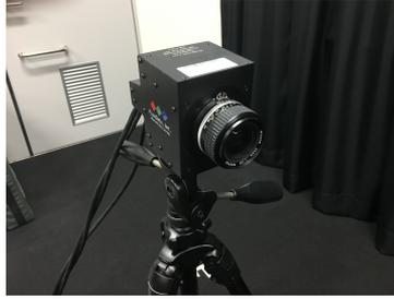
**Fig. 8** Polarization camera.
