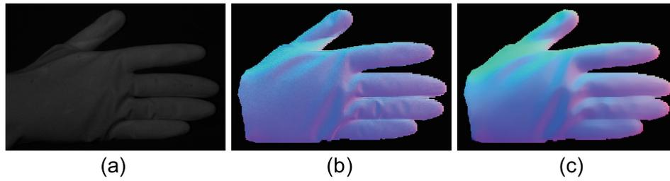
**Figure 25.** The result of hand with glove. Estimated surface normal [pose 1]: (a) One of the seven channel images, (b) estimated surface normal [naive color photometric stereo], and (c) estimated surface normal [our method]. Both color photometric stereos can estimate the surface normal of the dynamically deforming object.
