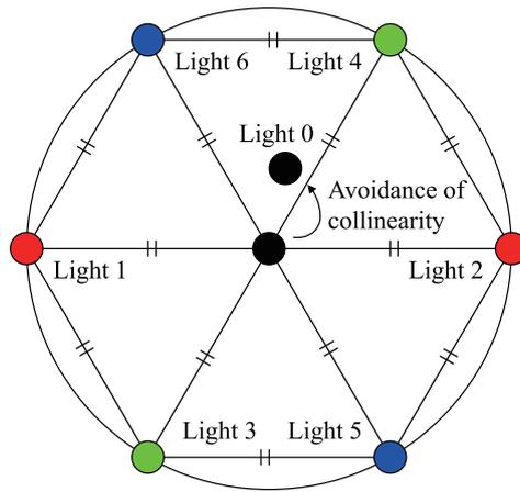
**Figure 12.** Schematic illustration of the geometrical location of seven light sources. Six lights are placed at each apexes of regular hexagon. Multispectral camera is placed at the center of the hexagon. Infrared light is placed near the camera.
