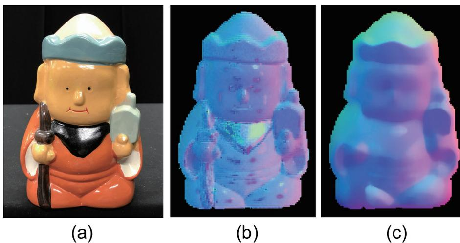
**Figure 22.** The result of buddha object, which causes strong specular reflection. Estimated surface normal [Buddha]: (a) Target object, (b) surface normal of naive color photometric stereo, and (c) surface normal of our method. The proposed method can smooth the surface normal of the scarf whose surface normal is unreliable due to black paint.
