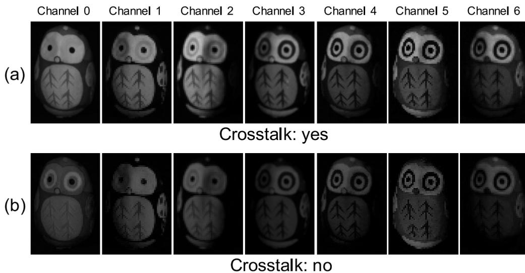
**Figure 15.** Obtained multi-band image [owl]: (a) Captured image and (b) image after cancelling channel crosstalk. If you look carefully, you may know that the channel crosstalk is removed. However, the difference is difficult to recognize since the crosstalk is small as is shown in Figure 9.
