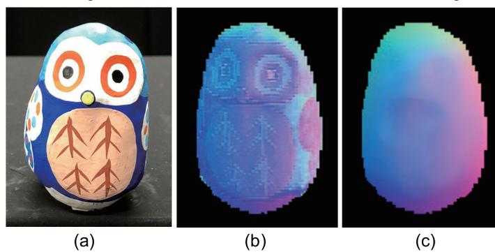
**Figure 16.** The result of owl object, which only causes diffuse reflection. Estimated surface normal [owl]: (a) Target object, (b) surface normal of naive color photometric stereo, and (c) surface normal of our method. The proposed method is not affected by the albedo difference.
