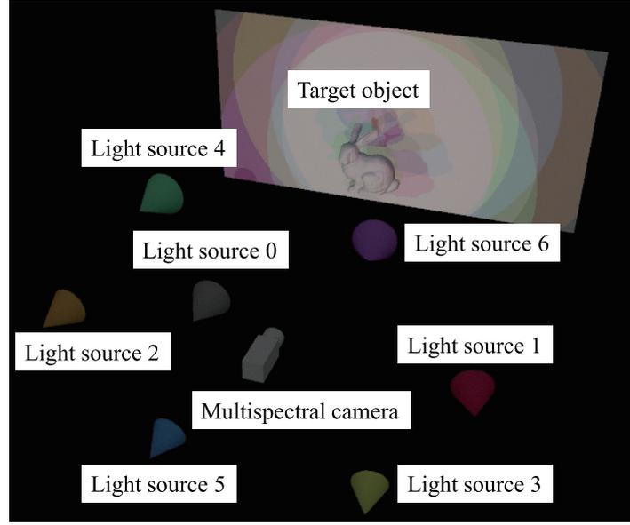
**Figure 1.** Conceptual explanation of multispectral color photometric stereo. Target object is illuminated by multiple light sources whose wavelengths are different. One image is taken using multispectral camera.
