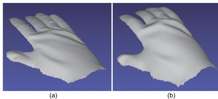
**Figure 27.** The result of hand with glove. Estimated geometry [pose 1]: (a) Estimated geometry [naive color photometric stereo] and (b) estimated geometry [our method]. Both color photometric stereos can estimate the surface normal of the dynamically deforming object.
