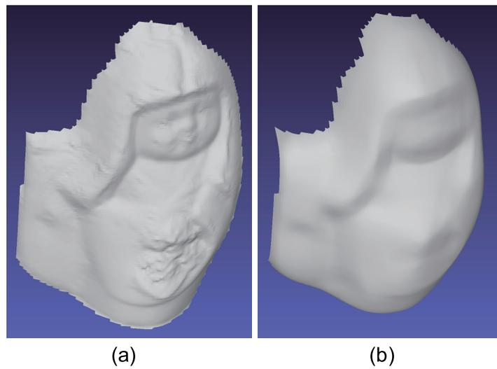
**Figure 21.** The result of doll object, which causes strong specular reflection. Estimated geometry [doll]: (a) Naive color photometric stereo and (b) our method. The proposed method is not affected by the albedo difference appears at the flower basket.
