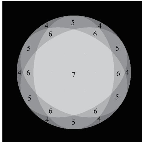
**Figure 11.** Gaussian sphere representation of surface normal where the north pole is the center of this picture. The number indicates how many light sources are lit for each direction of surface normal.
