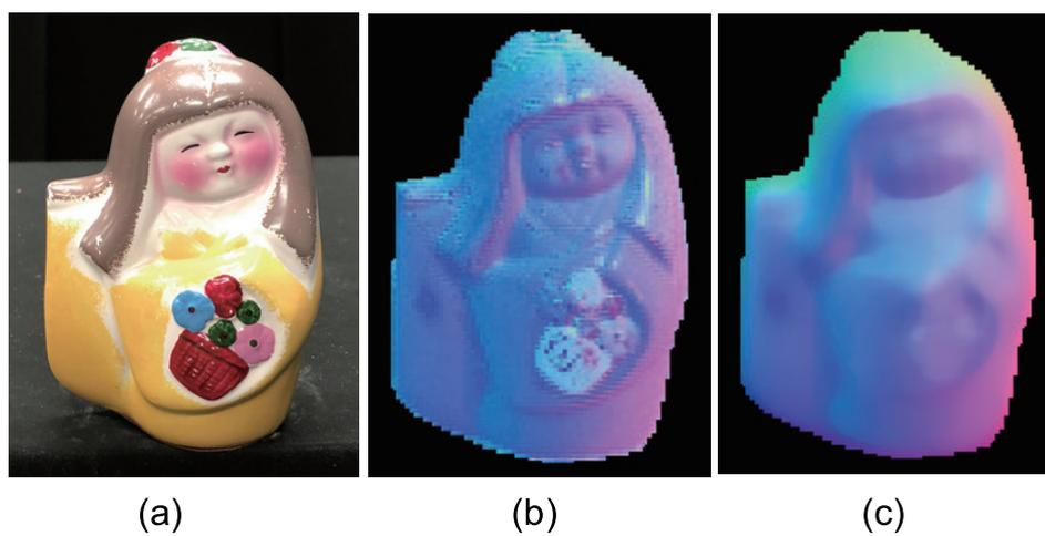
**Figure 19.** The result of doll object, which causes strong specular reflection. Estimated surface normal [doll]: (a) Target object, (b) surface normal of naive color photometric stereo, and (c) surface normal of our method. The proposed method is not affected by the albedo difference appears at the flower basket.
