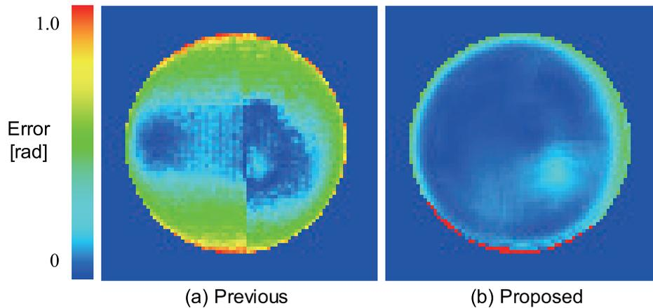
**Figure 14.** The error map of the sphere where the error is represented as angular difference between estimated value and ground truth (red: large, blue: small): (a) Naive color photometric stereo and (b) our method.
