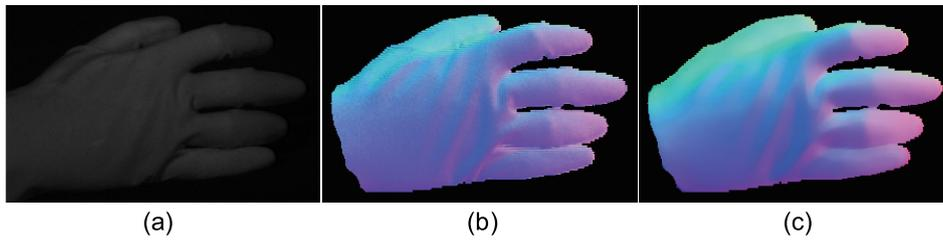
**Figure 28.** The result of hand with glove. Estimated surface normal [pose 2]: (a) One of the seven channel images, (b) estimated surface normal [naive color photometric stereo], and (c) estimated surface normal [our method]. Both color photometric stereos can estimate the surface normal of the dynamically deforming object.
