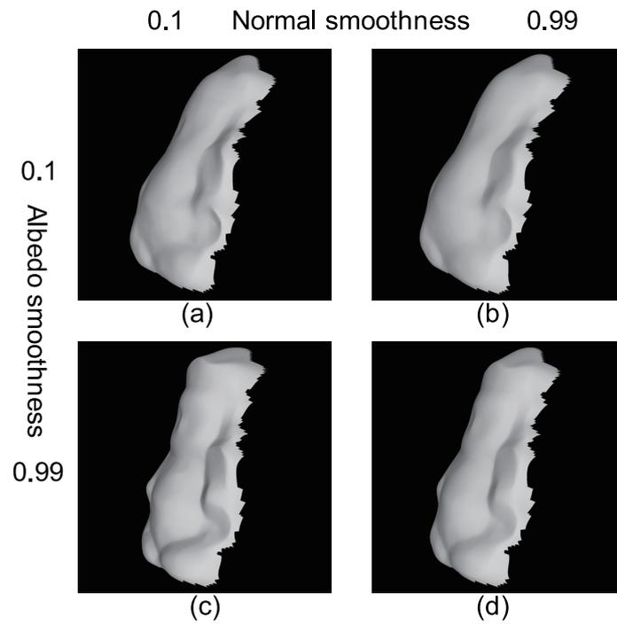
**Figure 32.** How the weight of smoothness term affects the results: (a) Sharp normal and sharp albedo, (b) smooth normal and sharp albedo, (c) sharp normal and smooth albedo, and (d) smooth normal and smooth albedo.
